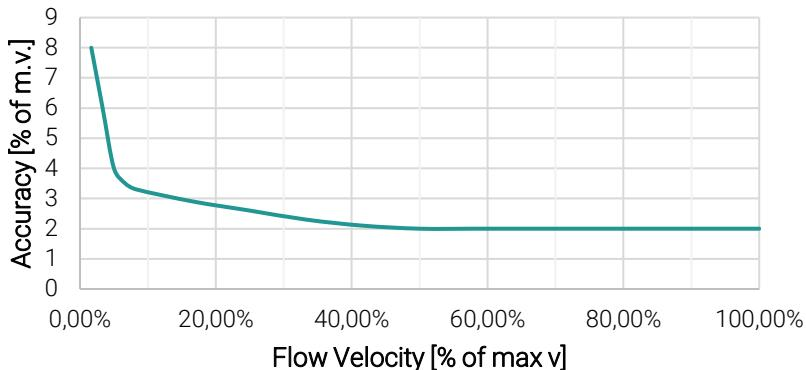
\* Accuracy specification per accuracy funnel, assuming turbulence-free flow conditions (refer to [installation notes](#)).
